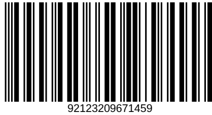
Figure 36: zint -b ITF14 --box --compliantheight -d "9212320967145"
