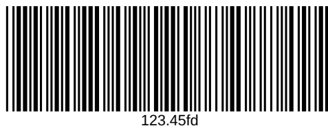
Figure 55: zint -b EXCODE39 --compliantheight -d "123.45$@fd"
