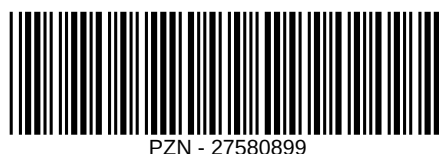
Figure 57: zint -b PZN --compliantheight -d "27580899"
