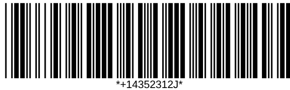
Figure 60: zint -b HIBC_39 --compliantheight -d "14352312"
