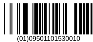
Figure 72: zint -b DBAR_OMN --complantheight -d "0950110153001"
