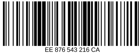
Figure 71: zint -b UPU_S10 --complantheight -d "EE876543216CA"
