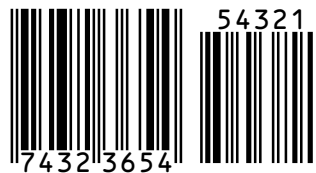
Figure 46: zint -b EANX --compliantheight -d "7432365+54321"
