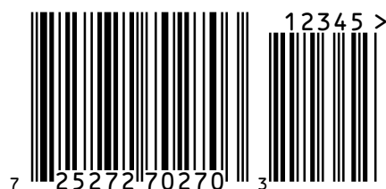
Figure 41: zint -b UPCA --complantheight -d "72527270270+12345" --guardwhitespace
