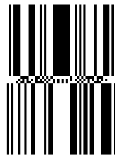
Figure 87: zint -b DBAR_OMNSTK --complantheight -d "9889876543210"
