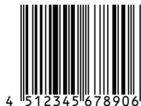
Figure 44: zint -b EANX --compliantheight -d "4512345678906"
