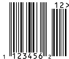
Figure 43: zint -b UPCE --compliantheight -d "1123456+12" --guardwhitespace
