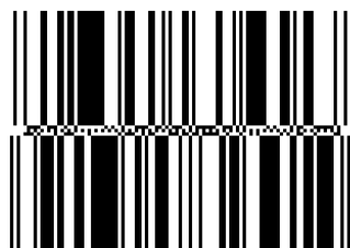
Figure 88: zint -b DBAR_EXPSTK --complantheight -d "[01]98898765432106[3202]012345[15]991231"
