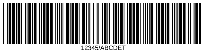
Figure 58: zint -b LOGMARS --compliantheight -d "12345/ABCDE" --vers=1
